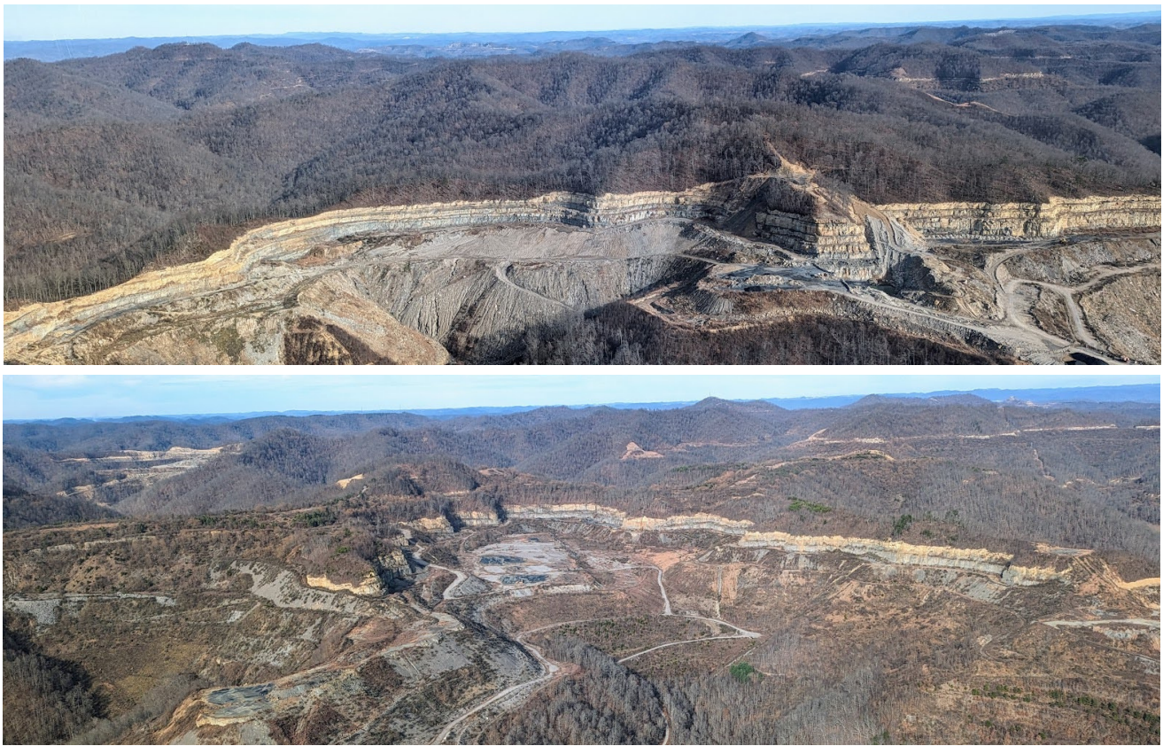
Figure 5: Photos taken in December 2023 of two mines permitted to Clintwood JOD, LLC. Images show thousands of feet of unreclaimed highwall. These mines have not produced coal since 2017 and 2019. Photo Credit: Appalachian Voices
